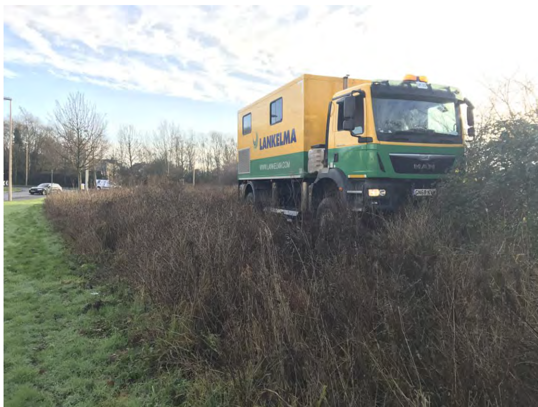
Plate 25. CPTu Tracked Truck in the position of CPT04
