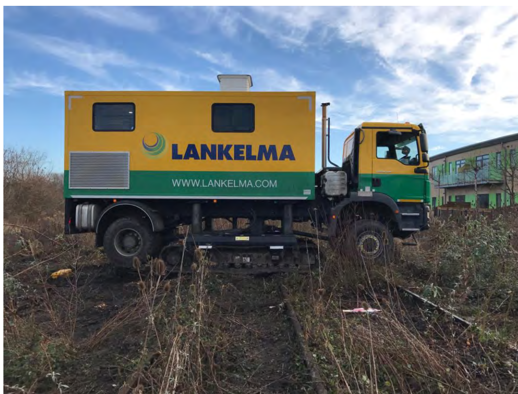
Plate 26. CPTu Tracked Truck in position of CPT05.
